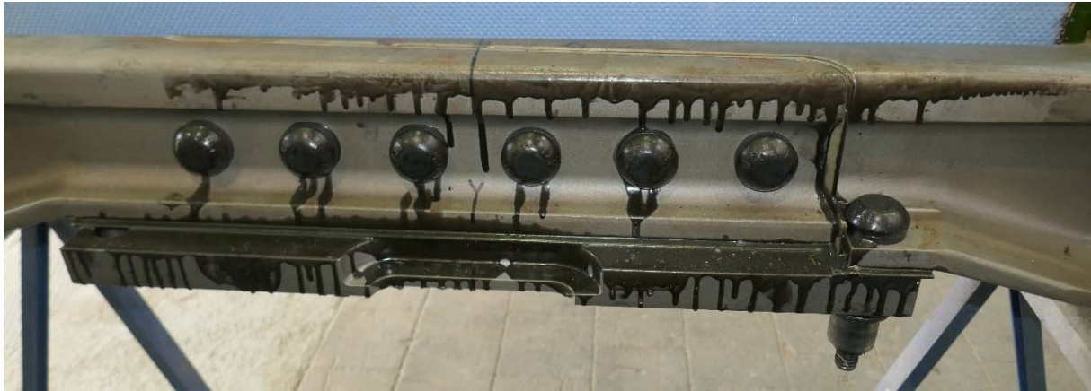
Figure 7: Opposite view of sample ABJ-009 after the bending fatigue test
