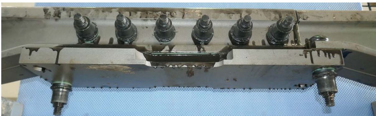
Figure 6: View of sample ABJ-009 after the bending fatigue test
