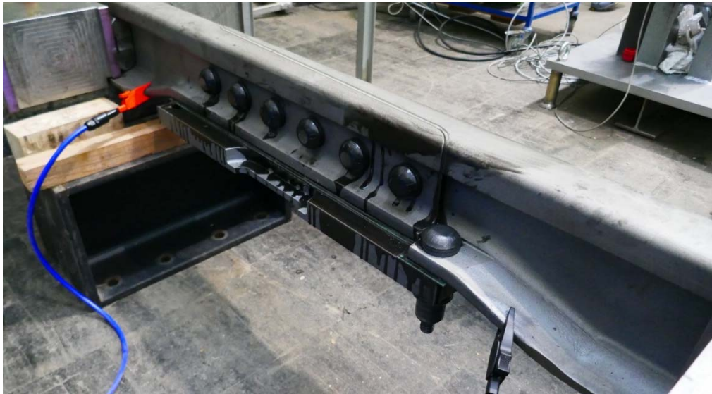
Figure 4: Sample ABJ-007 without damage after the tensile test (during the subsequent measurement of the insulation resistance)
