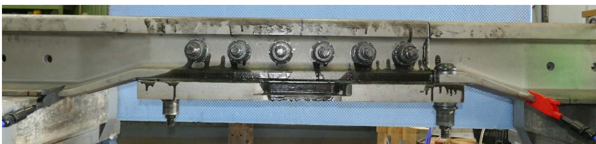
Figure 8: Measurement of insulation resistance on ABJ-009 after fatigue strength test
