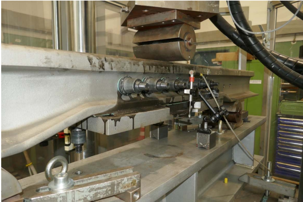
Figure 5: Sample ABJ-009 in the test setup of the 3-point-bending fatigue test
